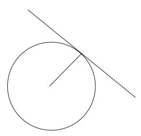
Angles between a tangent and its radius is always  $90^{\circ}$
